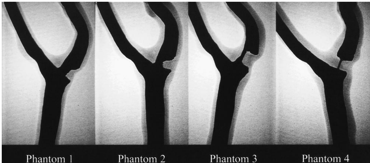
FIG 1. Digital radiographs of the iodinated contrast-material-filled carotid artery phantom models. The measured degree of stenosis is 38% for phantom 1, 61% for phantom 2, 80% for phantom 3, and 92% for phantom 4.
