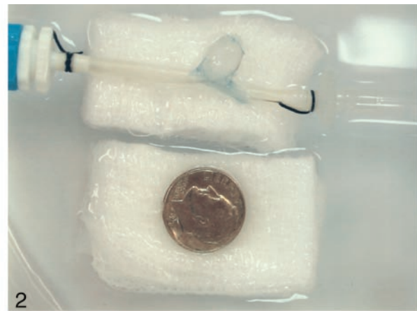
FIG 1. Vascular silicone phantom with a replica of the aortic arch, brachycephalic vessels, and a cerebral basin ( upper insert ). The systemic pressure could be adjusted by using a clamp on the main inflow vessel ( lower insert ).
