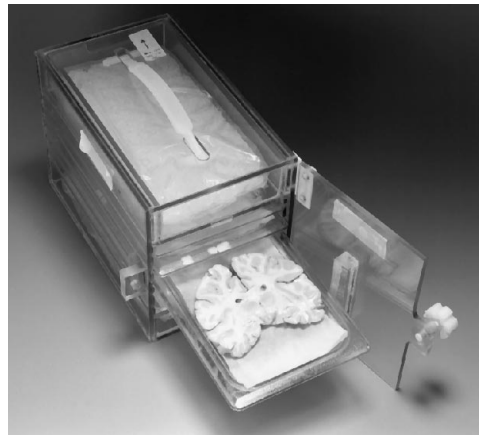
Fig 1. Brain slice holder with a brain slice on one of the five trays.
