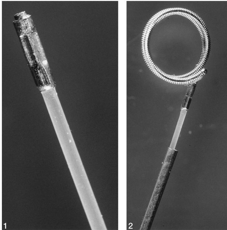
FIG 1. Laser probe. The laser fiber is produced by Trimadyne, Inc. The probe measures 300  $\mu$ m in diameter. The distal tip of the probe was milled in our institution's machine shop. A brass tip (3 mm in length  $\times$  0.6 mm in diameter) was crimped onto the distal end of the probe. The distal portion of the tip measures 0.2 mm in length  $\times$  0.3 mm in diameter.
