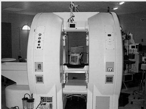
FIG 2. "Double donut" design is shown. General Electric Medical Systems Signa SP scanner consists of two very short superconducting cylindrical magnets separated by a 54-cm space to allow physician or nurse access. The space between the two magnet halves allows patient access from the top or sides, typically used with the surgeon and assistant on opposite sides of the patient's head. An optically linked frameless stereotactic tracking system is integrated into the top support piece. The scanner is designed for an operating-room environment, with electrical outlets and anesthesia gases integrated into the magnet covers. This system has a large fringe field, and all surgical instruments and accessory equipment in proximity to the system must be MR-safe or MR-compatible. (Photo courtesy of John Schenck, MD, PhD, and Robert W. Newman, MS, General Electric Medical Systems.)
