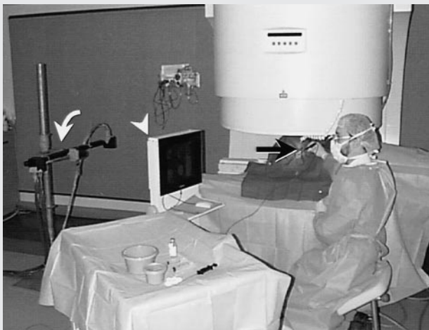
FIG 5. C-arm system for percutaneous intervention is shown. MR suite set up for radiologic intervention has three-camera video sensor array ( curved arrow ) that detects the location and orientation of a hand-held probe ( black arrow ). The system automatically acquires continuous MR images based on the probe position, and automatically updates display of four images on shielded LCD monitor adjacent to the scanner ( arrowhead ). A computer mouse on the LCD console and foot pedals ( not shown ) allow the scanner to be operated by the radiologist throughout the procedure.
