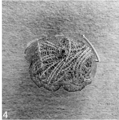
FIG 4. The liner, containing three coils, was retrieved from the in vitro aneurysm model. The first few millimeters of the first coil have penetrated the liner but the remaining coils are contained. The distal marker ring of the liner is visible as a dark dot in the upper third of the specimen.
