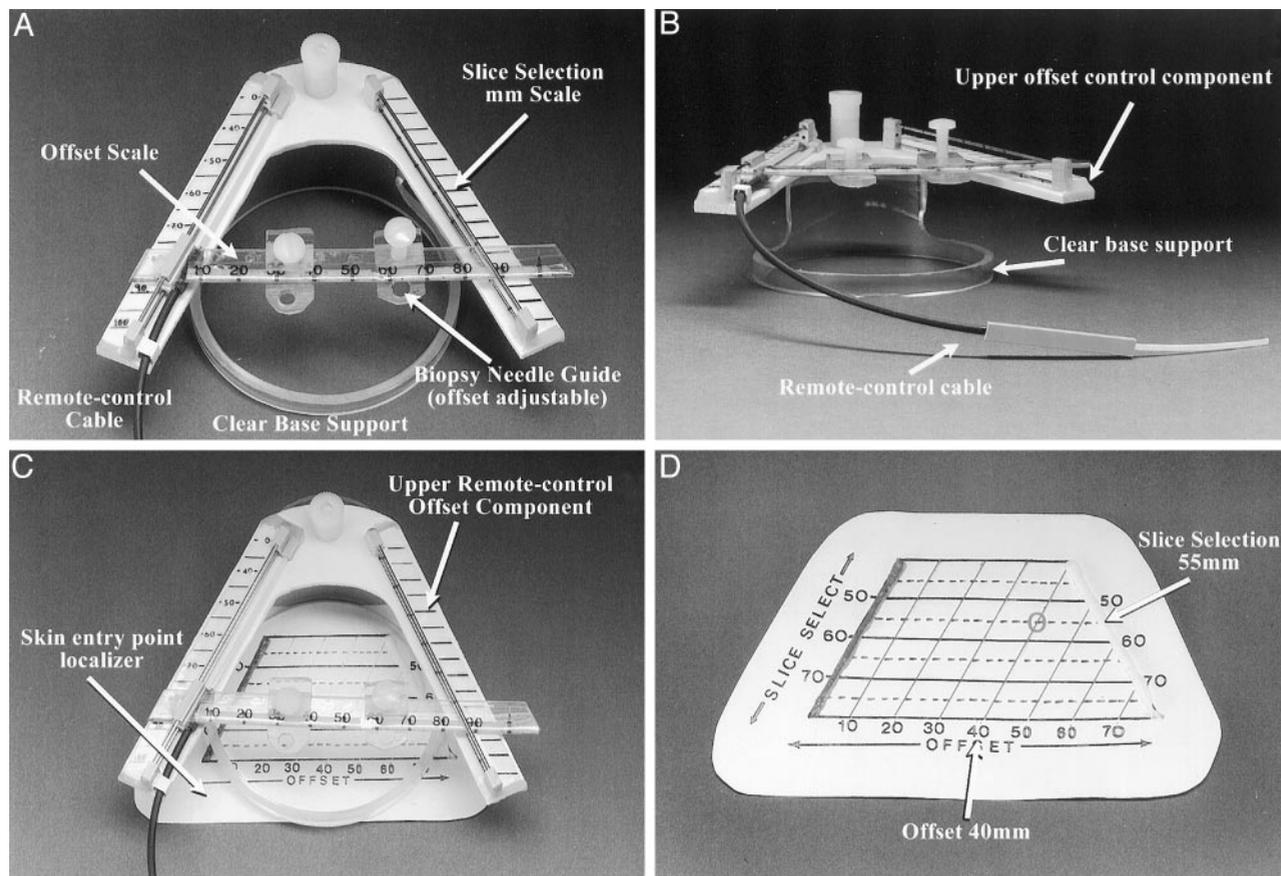
Fig 1. Components of the stereotactic CT navigator.
