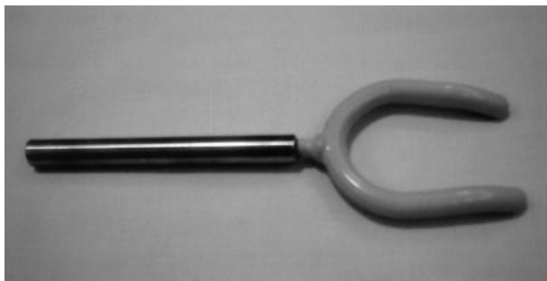
FIG 1. The prong deflector tool has an aluminum handle for operator grasp and control attached to a plastic covered steel two tine active end that is shaped to resemble the operator's fingertips with slight tine curvature and a 3–3.5-cm gap.
