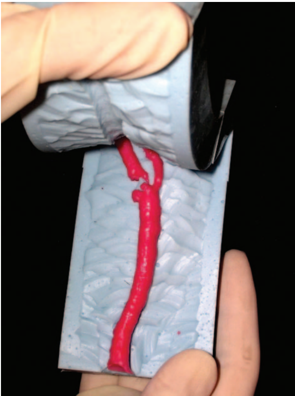
FIG 2. After reconstruction of the study segment on the Z Corporation RP machine, the plaster-like reproduction of the vessel lumen was used to make a master mold. Here the mold has been opened, revealing the wax model that reproduces the complex configuration and size of the original.
