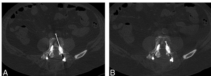
**FIG 2.** Extent of the flame artifact was quantified by measuring the distance (millimeters) from the tip of the metal object to the end of the linear dark band at the same level on both wFBP (A) and IMAR images (B). Improvement in artifact severity is demonstrated on the IMAR image.
