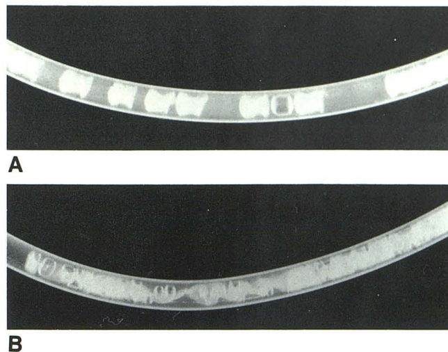
Fig. 3.—Appearance of bucrylate mixture after polymerization. A, Bucrylate mixture without acetic acid. After polymerization, it formed separate solid particles. B, Bucrylate mixture with acetic acid. After polymerization, it formed one long strand. Air bubbles result from delay between experimental work and photography.
