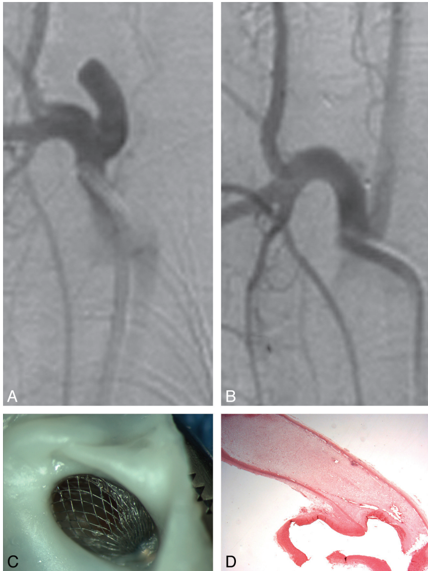
Fig 3. Representative images from case 2 in the Table. A , DSA before treatment shows the aneurysm. B , Image at sacrifice shows a small remnant at the neck. C , Gross examination shows the device is partially covered with membranous tissue, such that the aneurysmal cavity is open to the parent artery through the holes of the device. D , Photomicrograph of the aneurysm stained with H&E (original magnification = 12.5 \times ). The photomicrograph reveals thrombus at the neck, with no neointimal layer, and the remnant seen in B .
