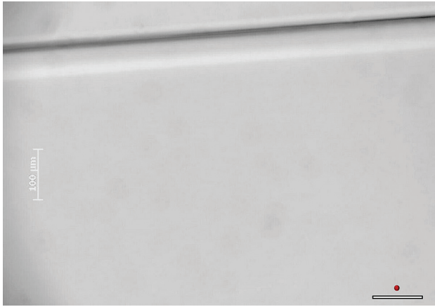
Fig 4. Freeze frame from On-line Video 5 of DSP flowing through a 200- \mu\text{m} -depth channel after mixing with LA and plasma. The straight line at the top of the image is the edge of the channel. No crystals or significant particulates are identified. The white scale bar in the bottom right of the image represents 100 \mu\text{m} . The adjacent red circle represents the average size of a RBC at this magnification. There is a separate scale bar on the left side of the image.
