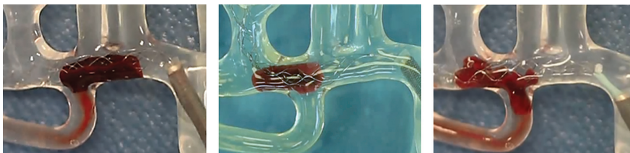
FIG 2. Clot types. The figure shows the 3 types of clot during MT inside the model: RBC-rich (left), fibrin-rich (middle), and hybrid friable clot (right).
