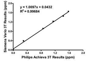
**ON-LINE FIG.** Cross-platform validation between Siemens Verio and Philips Achieva systems by using a ferumoxytol phantom.
