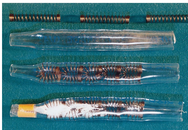
Fig 1. Model AVM nidus. The springs were forced into a U shape and pushed inside the Tygon tube successively. The bottom tube shows the PVAc precipitated inside the nidus. The white lines in the distal part of the tubes are artifacts of reflected light.
