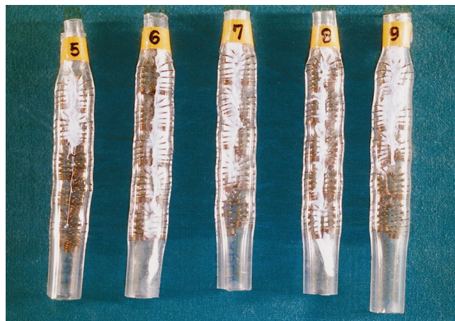
Fig 4. The precipitation of liquid PVAc plus metrizamide solution in the model AVM nidus at different flow velocities. Note that polymers remained inside the nidus at all flow velocities. No passage of threads was observed for this PVAc plus metrizamide solution. Precipitation behavior with the knob positioned at 3 and 4 was basically the same as that in Figure 3.
