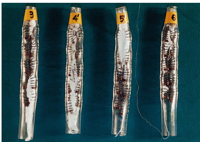
Fig 3. PVAc precipitated inside the model AVM nidus at different flow velocities. The numbers indicate the knob position on the peristaltic pump. PVAc precipitated outside the spring-filled region when the flow was slow (3 and 4'), but precipitated proximally when the flow velocity was increased (5'). With further increase in flow velocity, the polymer formed threads that passed the nidus (6).
