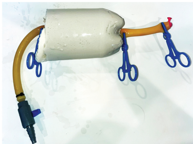
FIG 2. Constructed cervical phantom model. The photograph shows the fully-constructed phantom model. The cervical spine model is covered with polyalginate. There is a latex tube running through the spinal canal of the cervical model, with an inner latex balloon within the tube. The inner latex balloon is filled with dyed water, and the outer tube is filled with clear water. Two hemostats on either end of the phantom are occluding the posterior third of the latex tube to ensure that the balloon is in a more accurate anatomic position relative to the spinal cord. The hemostat at the distal end of the latex tube is used to maintain water pressure within the latex tube.
