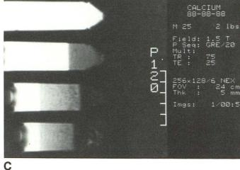
Fig. 2.—Experimental model of aqueous calcium phosphate solutions. Top tube contains pure water; salt content increases in each of the tubes below.
