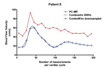
**On-line Fig 1.** Velocity data acquired by the ComboWire down-sampled to match the number of measurements obtained with PC-MR imaging compressed.
